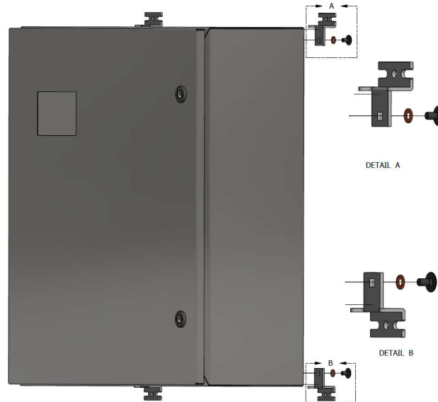
Figure 7 - Fitting the wall mounting brackets to the enclosure
