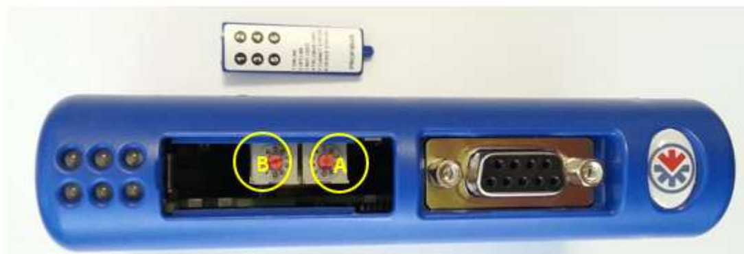
Figure 13 - Profibus module switch identification
