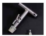
When either a 5 gram or 25 gram disposable En Core Sampler arrives at the laboratory, attach it to the Extrusion Tool, engage the plunger and push the sample into an appropriate vial.
